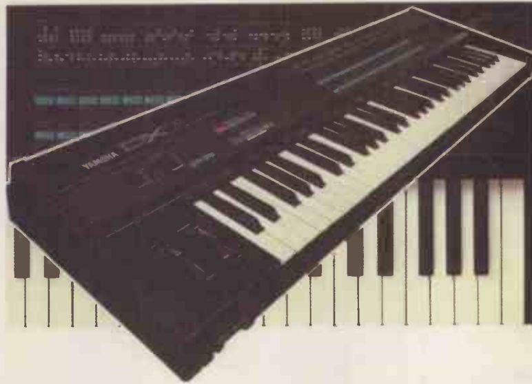
Fig. 8. Yamaha's DX7 – the first synthesiser to use frequency-modulation techniques.
