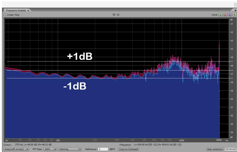
Even more interesting are the wideband, constant-velocity sweeps on CBS test record STR 120. These frequency sweeps (to 50kHz) allow us to see the enormous improvement the **PHLUX-AI** preamplifier wrings from a modest moving-magnet cartridge. The spectrogram of a recording of the L+R, 1kHz – 50kHz sweep is given below. The vertical white line defines the 20kHz point in the sweep.
