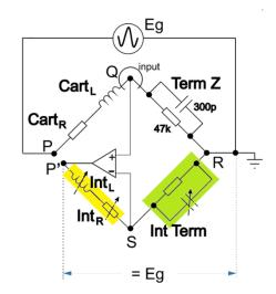
It is entirely possible to calibrate the bridge-balance by ear. In fact, this is an excellent approach. It should be noted, this is a *fine balance* adjustment, *the tonal differences* are subtle. There is no element of quality expressed in the control calibration: +4 is no better than -4. The numbers simply relate to the degree of adjustment from the nominal balance condition at the zero (12 o'clock) position.
