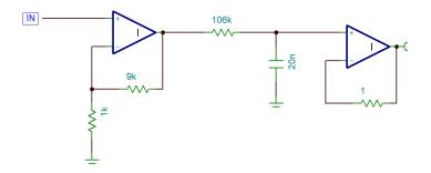
If we filter the OUTput noise with this filter and A-weight the result, the RMS noise falls to 98dB below calibrated maximum modulation (0.707V RMS) or -80dB below standard modulation level, an excellent figure, and one which betters most low-noise preamplifiers.
