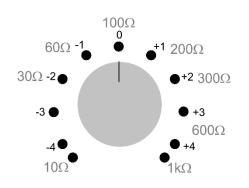
It is widely believed that input loading adjustment is worthwhile for moving-coil cartridges. To that end, when the **PHLUX-AI** preamplifier has the moving-coil front-end fitted, the bridge-balance knob controls the effect of the input loading on the cartridge by adjusting the mirror internal impedance of the Maxwell bridge.
