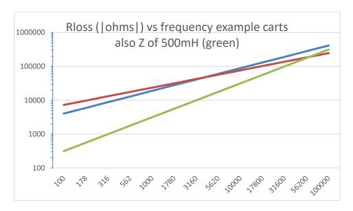
The practical implementation of this phenomena in the **PHLUX-AI** preamplifier is to account for the effect of  $R_{loss}$  only at the top of the audio band. (Its effect is relatively insignificant at lower frequencies, where  $R_{loss} >> |2\pi fL|$ ). The modulus of the impedance of a 500mH coil is given as the green line in the graph above.
