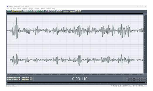
It seems therefore that, the "information" above 20kHz in the 96kHz needle-drop capture is largely a result of lower-frequency groove modulation provoking the inevitable resonance of the effective mass of the cartridge armature as it bounces on the compliance of the record material.
