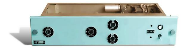
The Neumann WV2 is a vintage Zweikanal-Wiedergabeverstäker (two-channel playback preamplifier). The unit was originally designed for professional vinyl mastering and playback systems. Introduced in 1958, the WV2 was built for demanding, professional use and had a
