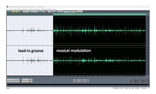
Clearly, these transients in the lead-in section were not part of the signal sent to the cutter head. One such lead-in "click" is illustrated below, with a magnification of the time axis sufficient to see the individual sampling points.
