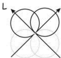
One way to improve the situation is to set the microphones at a greater angle than 90 degrees, or separate them slightly, so as to add a time-delay "helper" cue, as is done in the ORTF and NOS arrangements. But, it is also possible to correct for the effect of the unwanted, omni-response electrically; and that is what is done in the SHUpHLER when the switch is in the ♥ position.
