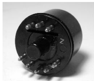
The VF14 tube used in the impedance converter of the U47
