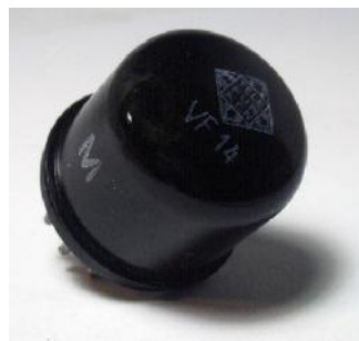
The VF14 tube used in the impedance converter of the U47
