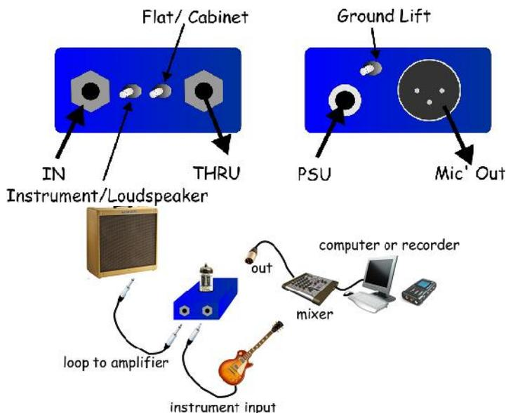
The Phædrus Audio PHI DI-Box is connected as shown in the diagrams above. Ensure that the "LOUDSPEAKER/INSTRUMENT" switch is in the "INSTRUMENT" position. However, note that feeding the output of the PHI into the studio console will negate some of the benefits of the PHI's unique character. Use a premium-quality microphone preamplifier (such as Phædrus Audio's PHAB) for the very best results as shown below.
