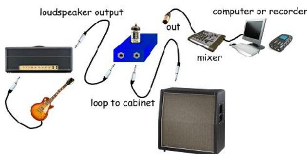
**YOU MUST SELECT THE "LOUDSPEAKER" POSITION OF THE LOUDSPEAKER/INSTRUMENT SWITCH WHEN CONNECTING THE Phædrus Audio PHI TO THE LOUDSPEAKER CIRCUIT OF AN AMPLIFIER. NOT SO DOING WILL DAMAGE YOUR Phædrus Audio PHI. FURTHERMORE YOU MUST OBSERVE THE WARNING GIVEN BELOW, AS FAILURE TO DO THIS COULD DAMAMGE YOUR AMPLIFIER.**
