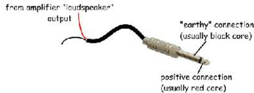
Furthermore, the Phædrus Audio PHI is NOT a dummy load and a loudspeaker MUST be attached to the THRU output so as to provide the correct load for the power amplifier. Valve amplifiers especially may be damaged without the correct speaker-load connected.
