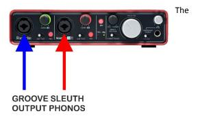
**Groove Sleuth Mk.II** is connected to your sound-card's line inputs (as shown above). Levels should be set on the interface in the normal way and you will find that the preamplifier delivers audio at a sufficiently high level for all commercial sound-cards, both internal and external.
