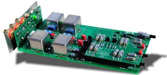
Recovery of the current-mode signal from the cartridge, suitably amplified for connection to a standard preamplifier or integrated amplifier is performed by the **PHATHOM** base-station (the interior of which is illustrated above). The design of this unit is simplified, in that no RIAA equalisation is included. But precision and very low-noise circuit techniques are required as the signal currents involved are very small (nano-amperes).
