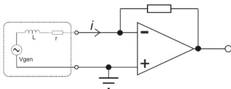
Now, at this point, it would be reasonable to ask: what's the use of a transducer with short-circuited terminals. How do you get the signal out? The circuit above illustrates how this current may be detected and amplified. Here, the cartridge feeds a *trans-resistance* or *trans-impedance* preamplifier. The amplifying action of the amplifier and the feedback resistor hold the inverting input (-) at the same potential as
