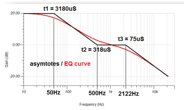
The specification of the RIAA tone-control was standardised for all records from 1955: the parameters are illustrated in the graph.
